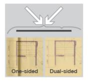
Contex CleanScan CIS The IQ Quattro Scanners are equipped with Contex CleanScan CIS modules which facilitate optical image quality with dualsided LED lighting. This eliminates creases and folds in originals normally a challenge for CIS scanners, and thus provides clear, crisp scans every time.
