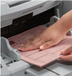
For enhanced reliability, staple detection sensors are also incorporated to help prevent any damage to documents, while a continuous manual feeding mode allows convenient controlled feeding to users when handling difficult documents. Lockable paper side guides also ensure smooth, productive scanning.
