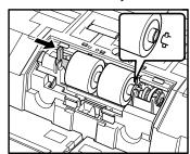
7. Pull the roller lock lever down to lock the retard roller in place.
