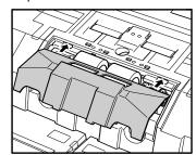
**9.** Push the front of the roller cover in. Check that it makes a latching sound and that it is securely returned to its original position.
