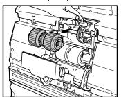
**5.** Open the roller holder, and insert the new pickup roller.
