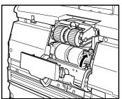
**9.** Close the roller cover. Check that it makes a latching sound and that it is securely returned to its original position.
