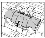
10. Gently lower the upper unit (1). Press down on both sides of the upper unit to ensure that it is securely closed (2).
