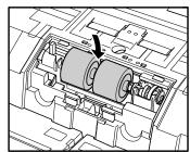
**6.** Align the notches in the roller with the shaft pins in the scanner, then slide the roller lock lever in the direction indicated by the arrow.
