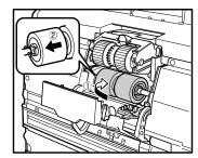
8. Push the roller lock lever up to lock the feed roller.
