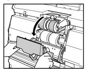
3. Pull the roller lock lever down.
