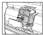
6. Place the new feed roller on the pin.
